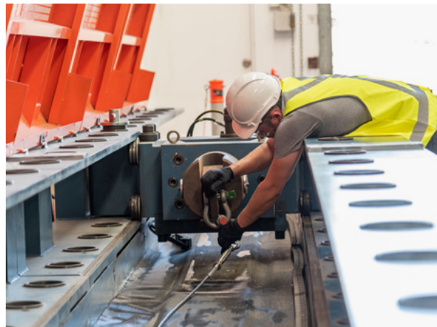
Wire Rope testing on 300t Test Bed
